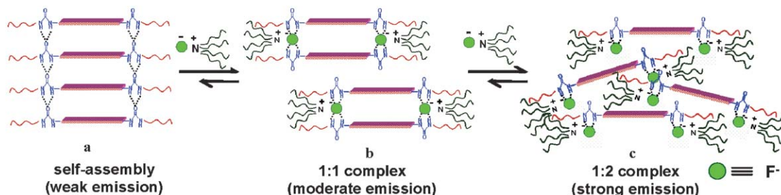
Fig. 3 Interaction of F^- with the BU-OPV1 self-assembly which justifies the enhancement in fluorescence.
